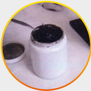
Heavily hydrocarbon/mineral oil contaminated sample (T-zero, as received for analysis).
